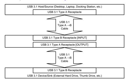
Figure 1. TUSB214 Functional System Level Block Diagram
