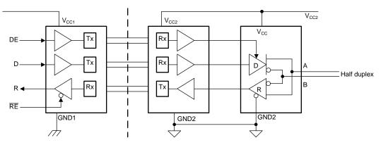
Figure 1. ISO1500DBQ Functional Block Diagram
