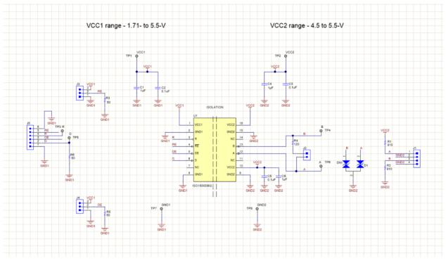
Figure 5. ISO1500DBQ Schematic
