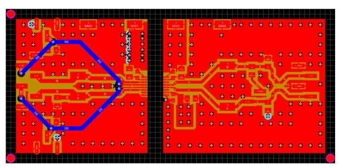
Figure 4. Signal-Layer View Half Duplex Isolated RS-485 EVM
