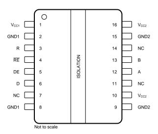
Figure 2. ISO1500 DBQ Package 16-Pin Configuration
