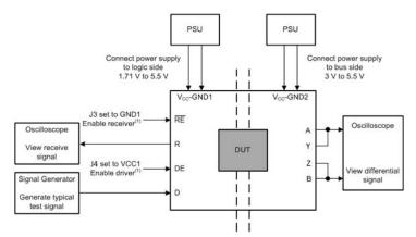
(1) Normal transceiver operation requires both the driver and the resections to be active. Set the enable pin (RE) to logic low and the driver enable pin (DE) to logic high.
