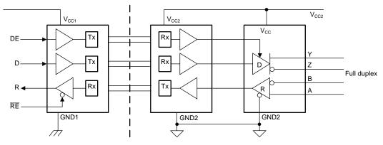
Figure 1. ISO1412 Functional Block Diagram
