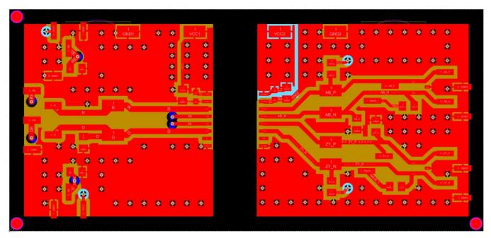
Figure 4. Top-Layer View Full Duplex Isolated RS-485 EVM
