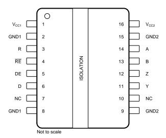
Figure 2. ISO1412 DW Package 16-Pin SOIC Pin Configuration
