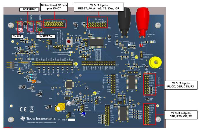
Figure 2. 5.5 V to 3.3 V interface image
