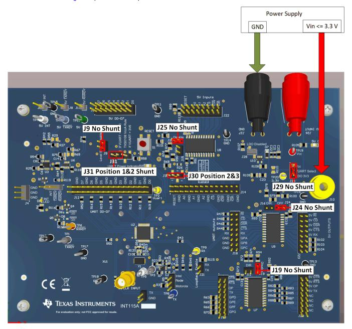
Figure 5. DUT below 3.3 V
