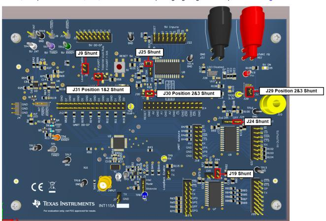
Figure 1. High to low shunt image
