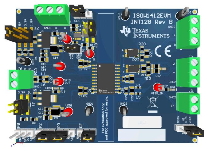
Figure 4-1. ISOW1412DFMEVM PCB 3D diagram
