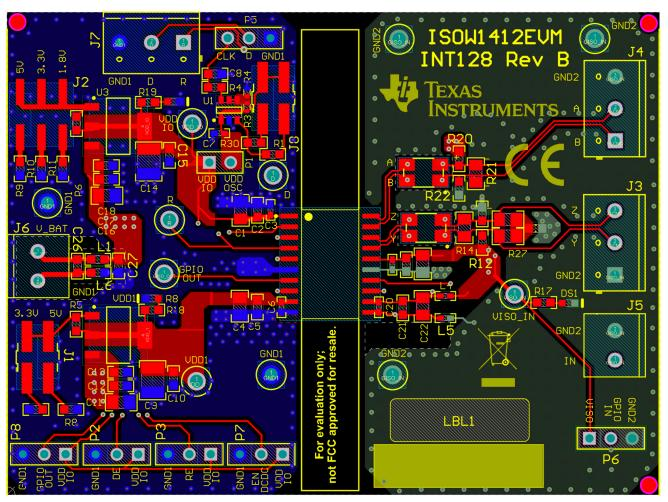
Figure 4-2. ISOW1412DFMEVM PCB Layout - Top Layer
