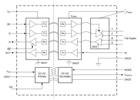
Figure 2-1. ISOW1412 Functional Block Diagram
