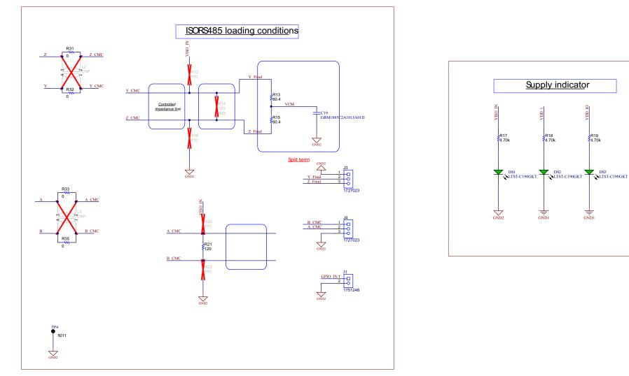
Figure 3-3. ISOW1412DFMEVM Schematic - RS-485 Bus
