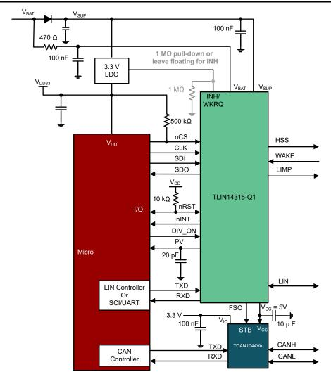
Figure 2-4. Channel Expansion with CAN Transceiver
