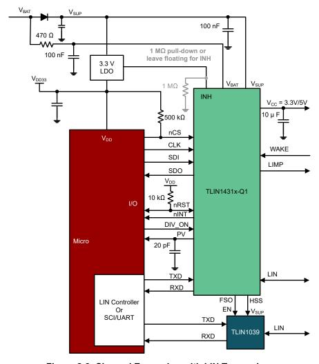
Figure 2-3. Channel Expansion with LIN Transceiver
