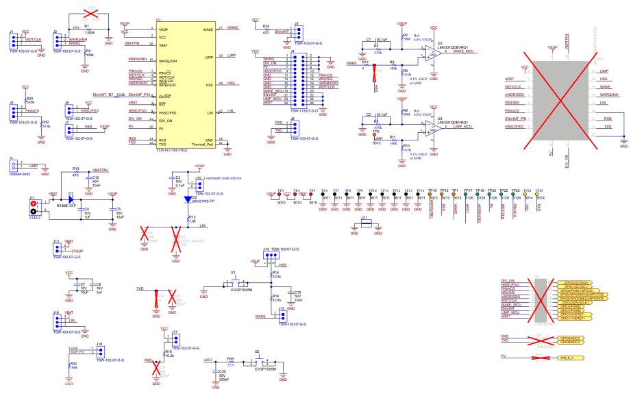
Figure 5-1. TLIN1431EVM Schematic
