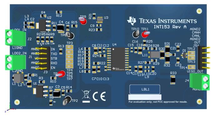
Figure 6-3. ISOW1044DFMEVM PCB 3D Diagram
