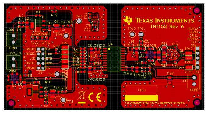
Figure 6-1. ISOW1044DFMEVM PCB Layout - Top Layer
