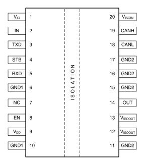
Figure 3-1. ISOW1044 Isolated CAN Transceiver with Integrated DC-DC Converter Pin Configuration
