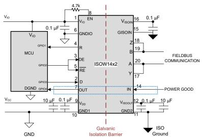
Figure 8. Use of GPIO channel for diagnostic signal transfer
