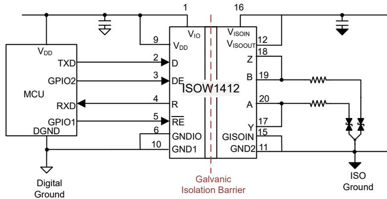
**Figure 2. Integrated implementation of isolated RS-485 and isolated power**
