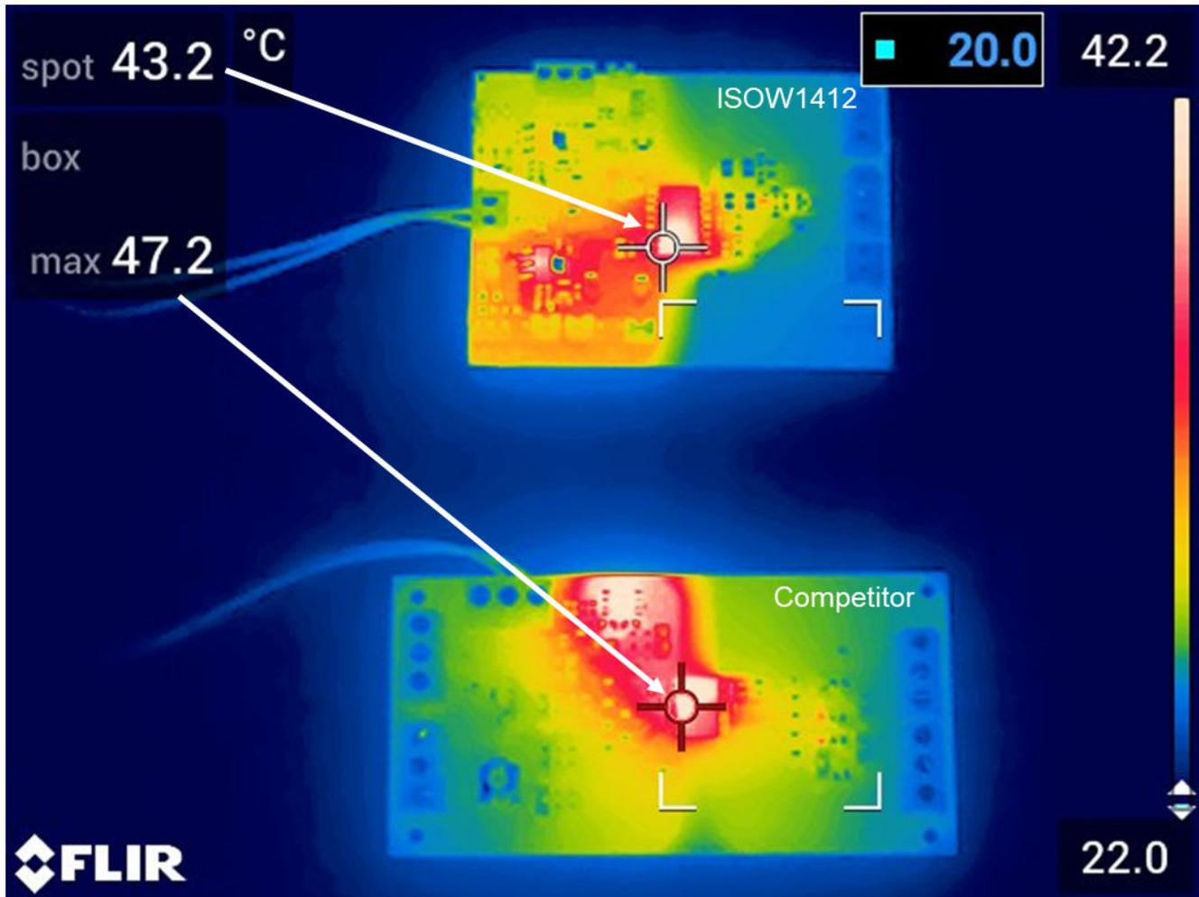
**Figure 5. Thermal comparison between ISOW1412 (top) and leading competitor (bottom) for 5 V Vin and Vout with 60-Ohm RS-485 termination**
