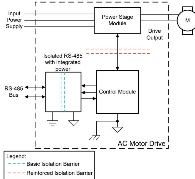
**Figure 6. Typical block diagram of AC Motor drive**
