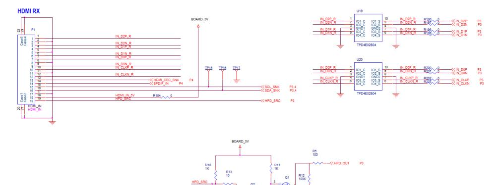
Figure 4-2. HDMI Input Connector
