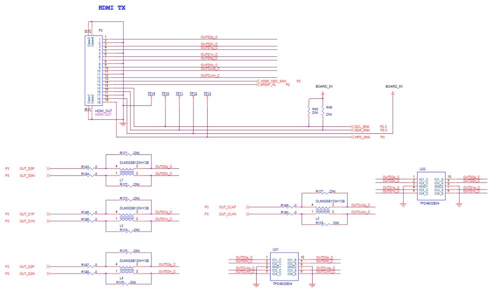
Figure 4-4. HDMI TX Connector
