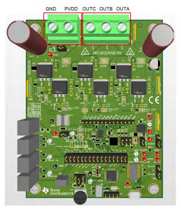
Figure 4-2. Connections from Motor to MCT8329EVM
