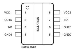
Figure 2-1. ISO6521 Functional Isolator Pin Configuration
