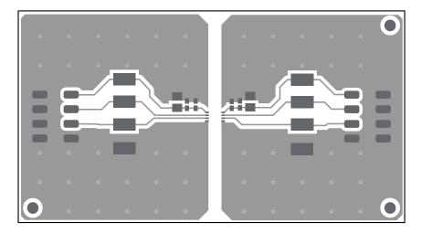
Figure 3-3. ISO6521REUEVM PCB Layout - Top Layer
