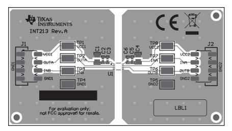
Figure 3-2. ISO6521REUEVM PCB Layout - Composite Top View
