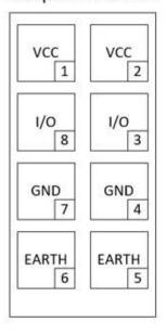
Figure 2-1. Single Ended (Console Side) Jumper Map
