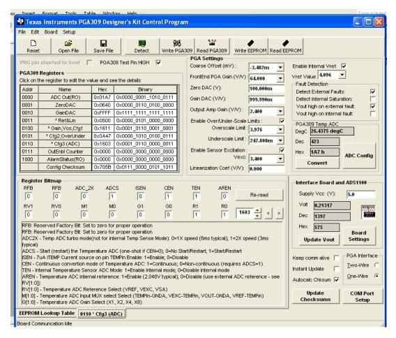
Figure 21: PGA309 Registers - Main Window
