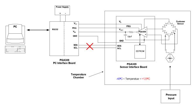
Figure 46: Use One-Wire (PRG) Interface for Temperature Calibration
