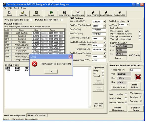
Figure 9: Software Startup - Wrong Com Port
