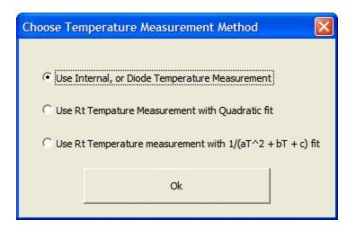
Figure 40: Choose Temperature Calibration Method
