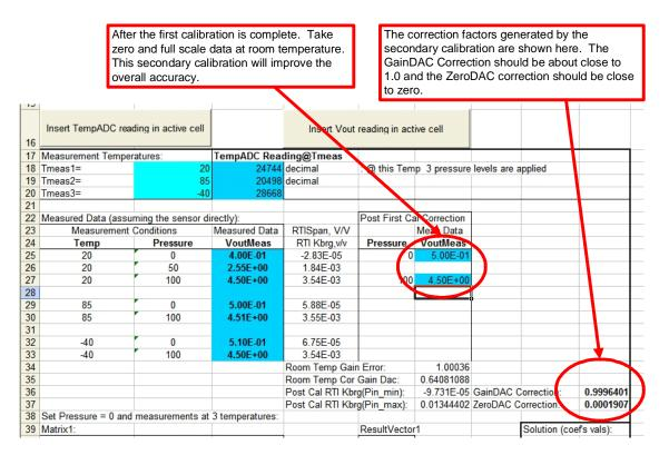
Figure 44: Second Calibration for Improved Accuracy.
