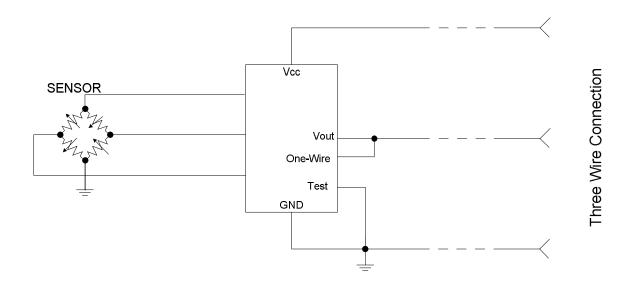
Figure 28: Three Wire Configuration
