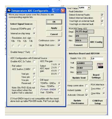
Figure 22: PGA309 Temp ADC Configuration & Readback
