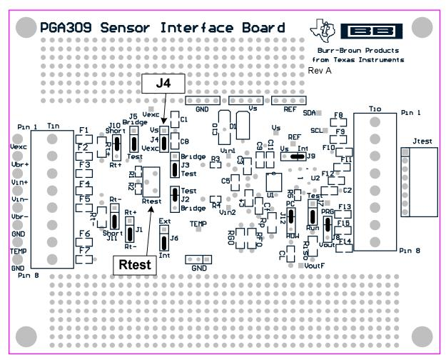
Figure 3: PGA309 Sensor Interface Board – Factory Jumper Settings
