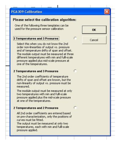
Figure 39: Select Calibration Algorithm Dialog
