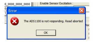
Figure 45: "Read ADS1100 Continuously" Error Message
