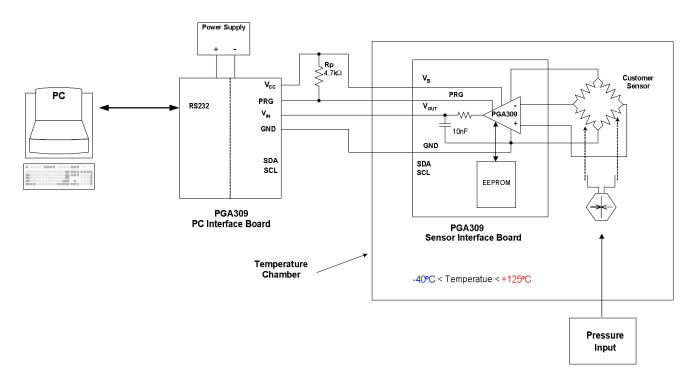
Figure 47: PGA309 4-Wire Sensor Module Application
