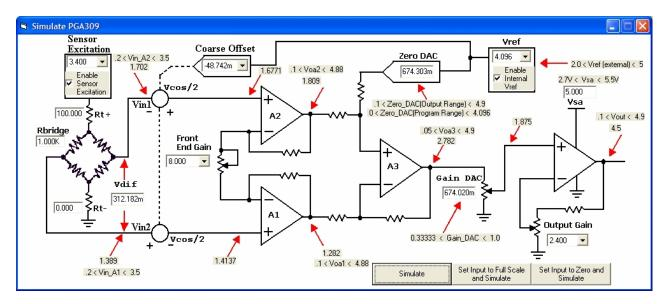
Figure 33: Simulate PGA309
