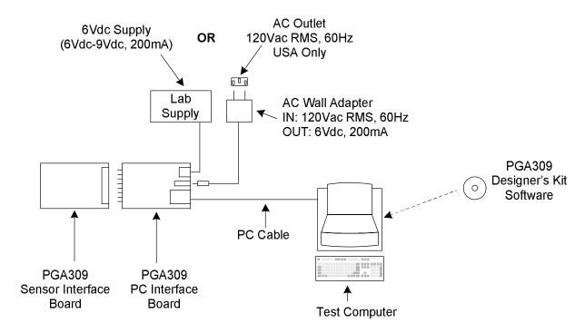
Figure 5: Hardware Setup - Initial Checkout
