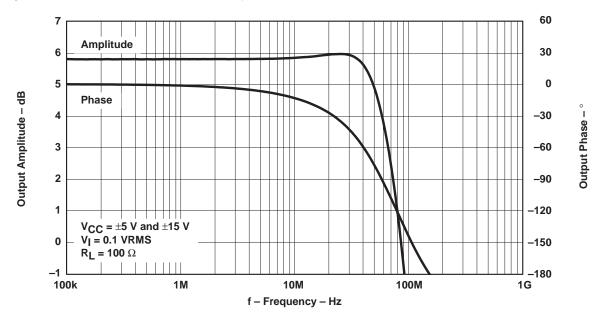
Figure 1–3. THS4081 EVM Frequency Response With Gain = +2
