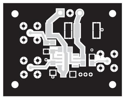
Figure 2–2. THS4081 EVM PC Board Layout: Component Side
