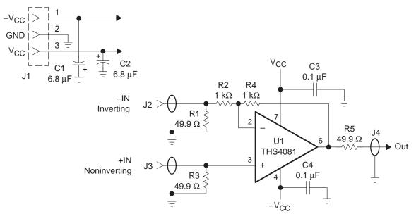
The gain of the EVM inputs can easily be changed to support a particular application by simply changing the ratio of resistors R1, R4, and R5 as described in the following equations:
