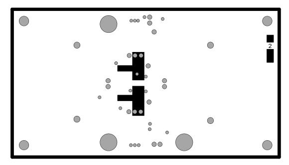
Figure 1–10. Internal Plane (Layer 3) (± Power Plane)
