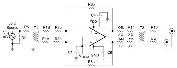
**Note:** Utilizing the input and output transformers to create a fully-differential signal input/ differential or single output and isolate the amplifier from the rest of the front-end and back-end circuits.
