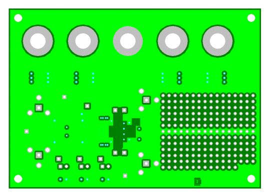
Figure 4-3. Internal Plane (Layer 3) (Power Plane)
