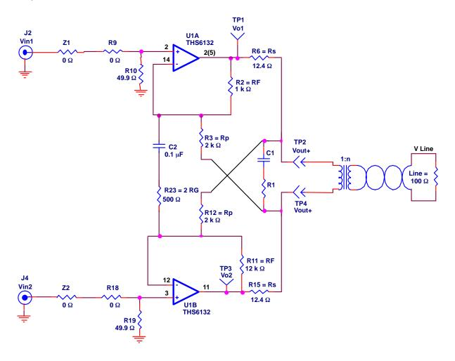
Note: Component pin numbers shown are for THS6132RGW while pin numbers in parentheses are for THS6132VFP.
