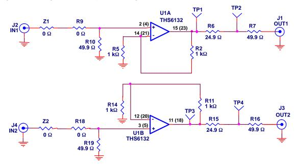
Figure 3-5. Single-Ended Amplifier Configuration
