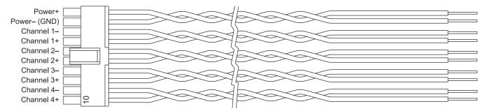
Figure 1-3. Wiring Harness for Power and Speaker Connections
