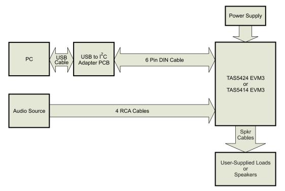
Figure 1-4. EVM System Connection Diagram
