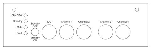
Figure 1-1. End Panel for Input Connections
