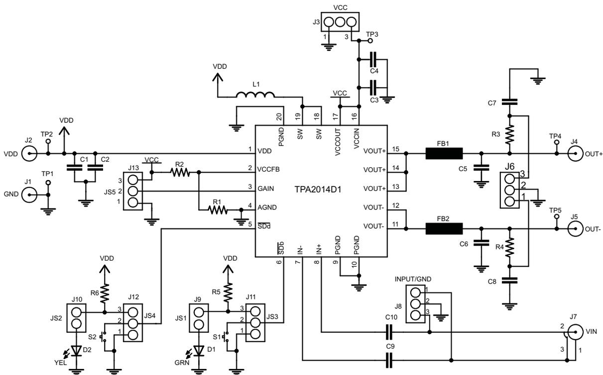
Figure 1. TPA2014D1EVM Schematic
