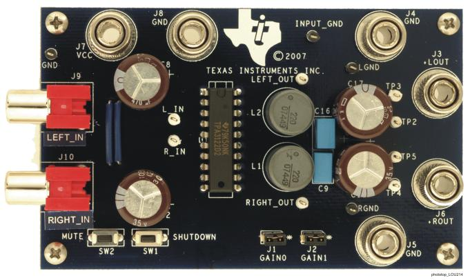
Figure 1. TPA3122D2 Audio Power Amplifier EVM - Top View
