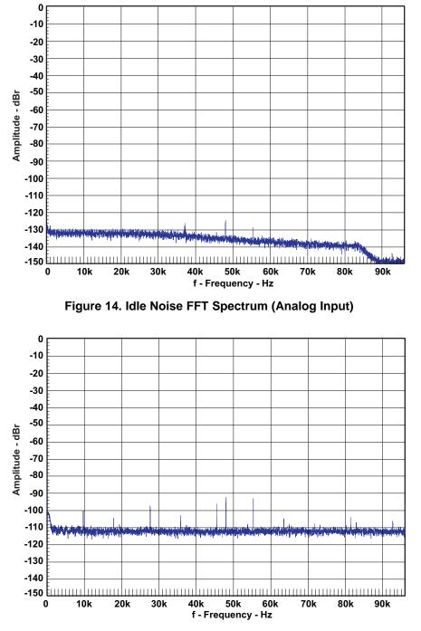
Figure 15. Idle Noise FFT Spectrum (Digital Input)
