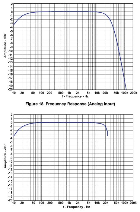
Figure 19. Frequency Response (Digital Input)
