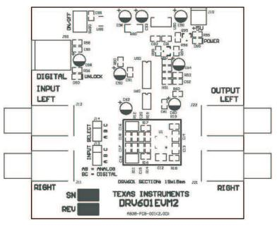
Figure 22. DRV601EVM2 PCB Component Placement Top
