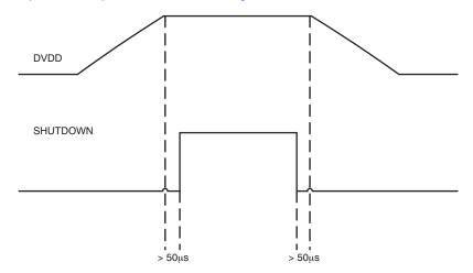
Figure 4. Power-Up/Down Sequence
