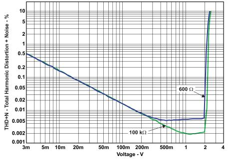
Figure 6. THD+N vs Voltage (Analog Input)
