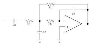
Figure 5. Second-Order, Active Low-Pass Filter
