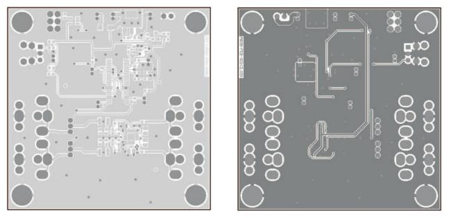
Figure 23. DRV601EVM2 PCB Top and Bottom Layers
