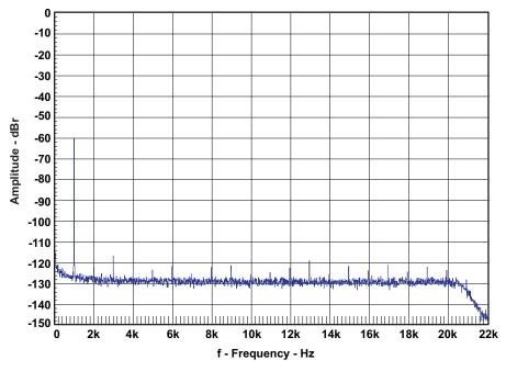
Figure 13. FFT Spectrum With -60-dBFS Tone (Digital Input)
