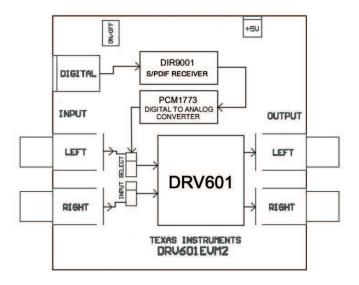
Figure 2. DRV601EVM2 Functional Block Diagram
