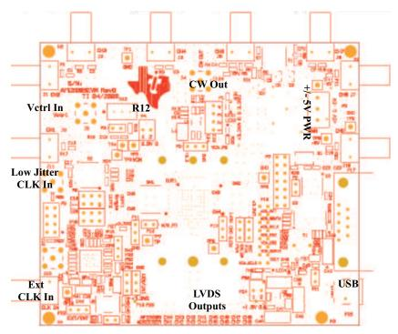
Figure 2. AFE5805EVM I/O Connectors and Locations
