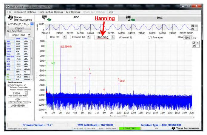
Figure 28. Typical Performance of AFE5805 in Non-Coherent Case
