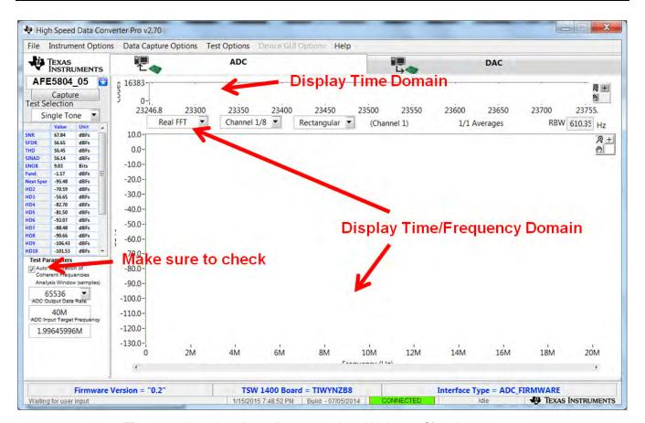
Figure 24. User Interface: Frequency Load Value to Signal Generator
