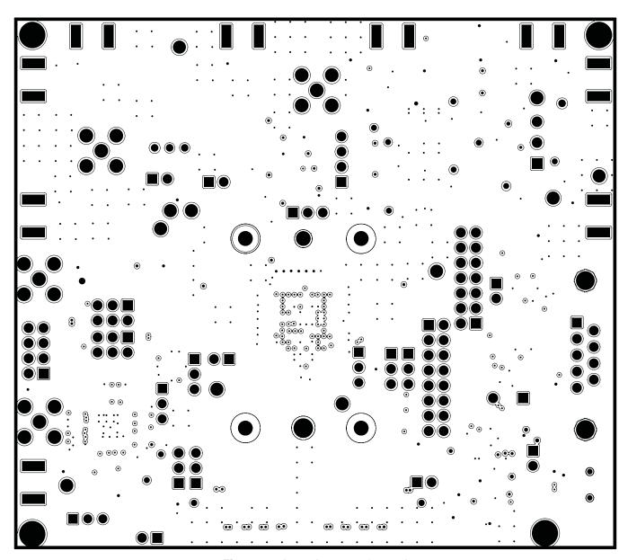
Figure 11. Inner Layer 1, Ground
