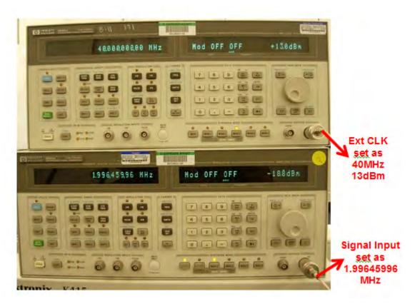
Figure 21. Connection of the Instruments
