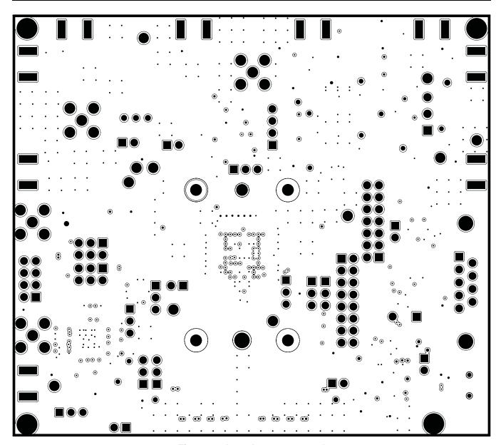
Figure 14. Inner Layer 4, Ground
