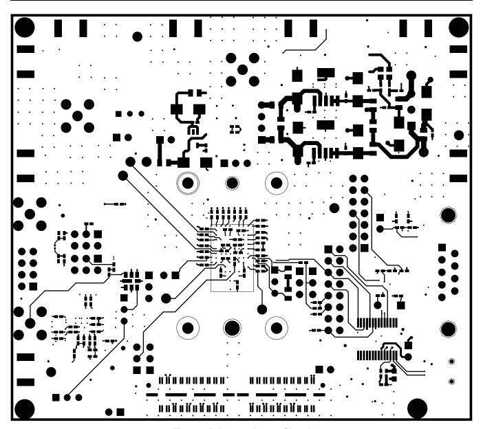
Figure 15. Bottom Layer, Signal
