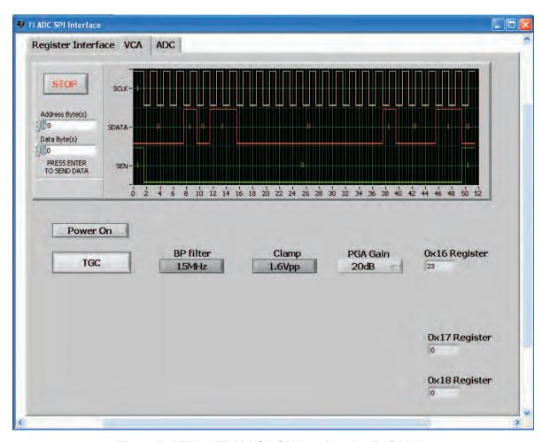
Figure 5. AFE5805EVM USB SPI Interface for TGC Mode
