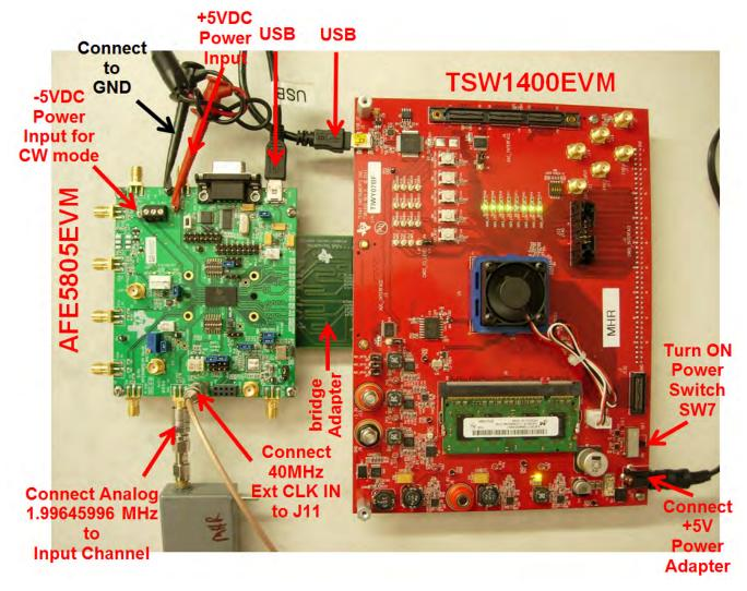
Figure 20. Connection between TSW1400EVM and AFE5805
