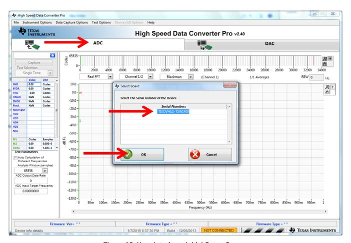
Figure 35. User Interface: Initial Setup Screen
