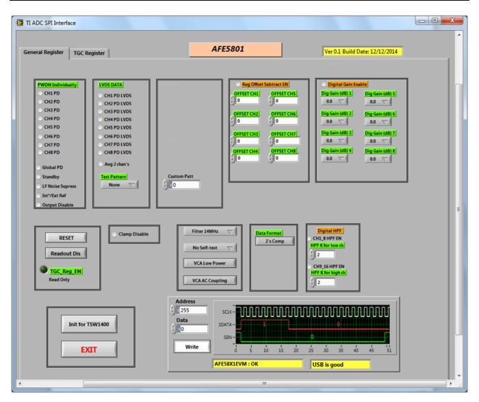
Figure 31. AFE5801EVM GUI - RUN Mode
