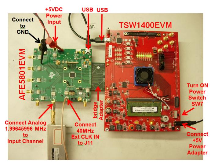
Figure 29. Connection Between TSW1400EVM and AFE5801
