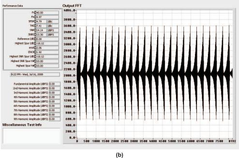
Figure 28. Typical Performance of AFE5801. (a) Fixed Gain Mode; (b) Variable Gain Mode
