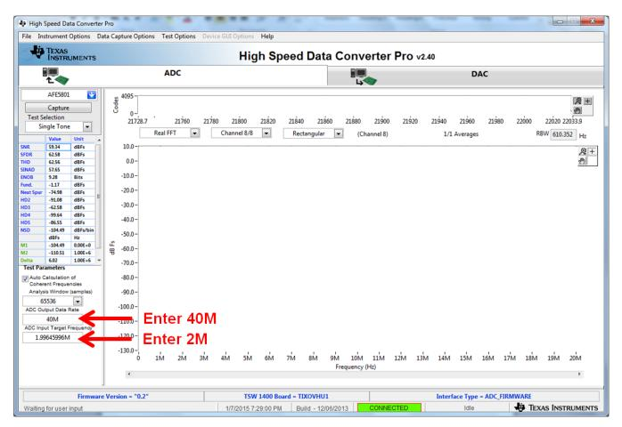
Figure 37. User Interface: Frequency Load Value to Signal Generator
