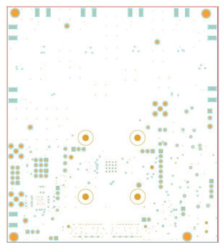
Figure 24. Inner Layer 4 Ground
