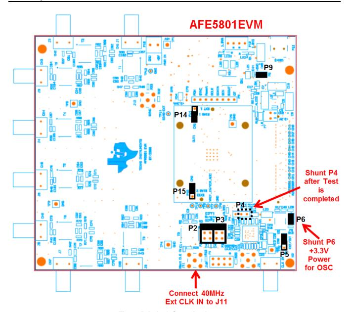
Figure 5. Default Setup for Jumpers
