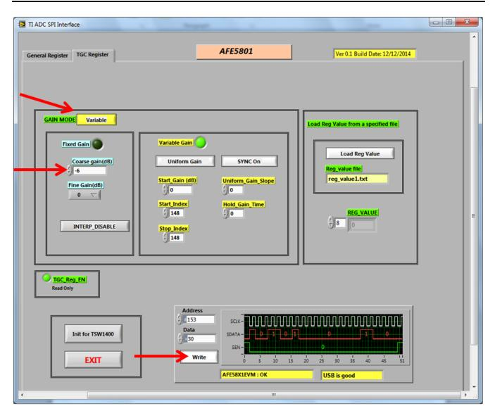
Figure 33. AFE5801EVM GUI - Variable Gain
