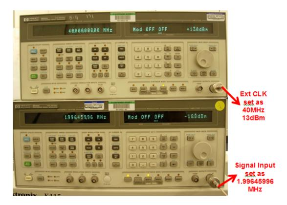
Figure 30. Connection of the Instruments
