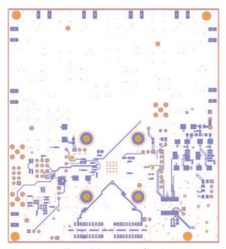
Figure 25. Bottom Layer Signal
