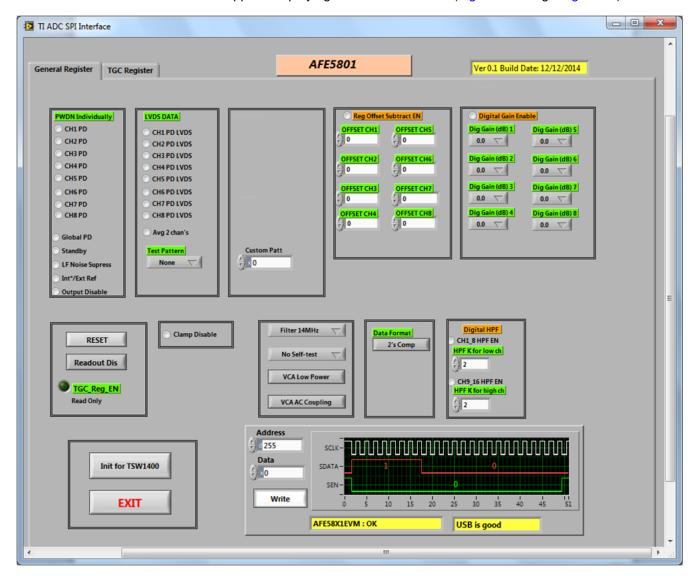
Figure 9. AFE5801EVM USB SPI Interface for General Registers.
