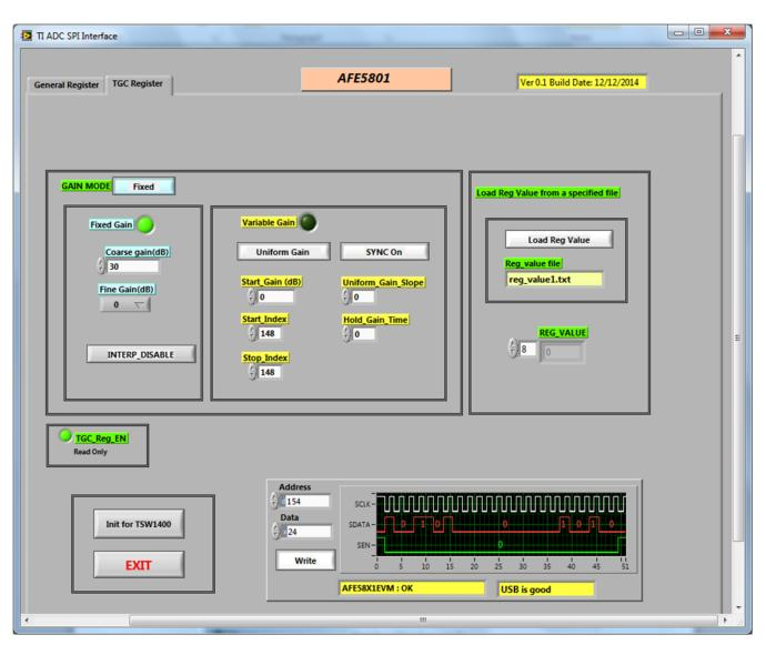
Figure 10. AFE5801EVM USB SPI Fixed Gain Mode
