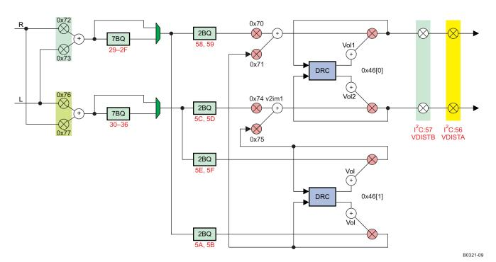
Figure 6. Process Flow for TAS5707 UG
