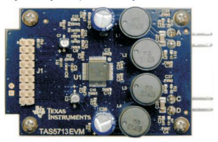
Figure 1. TAS5713EVM Printed-Circuit Board
