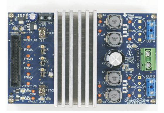
Figure 1-1. The TI DRV8432EVM Motor Drive Evaluation Board – Top View
