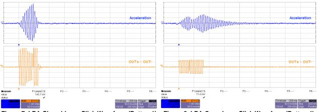
Figure 7. LRA Closed-Loop Click Waveform (Button 1) Figure 8. LRA Open-Loop Click Waveform (Button 4)
