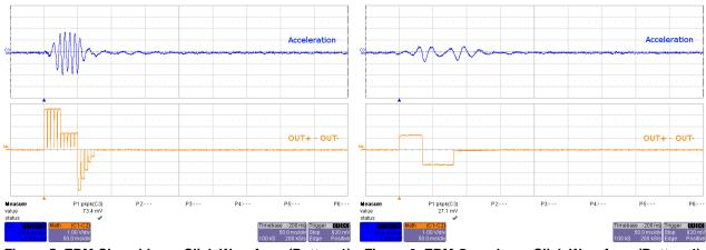
Figure 5. ERM Closed-Loop Click Waveform (Button 1) Figure 6. ERM Open-Loop Click Waveform (Button 4)
