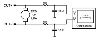
Figure 22. Measuring the DRV2604 Output Signal with an Analog Low-Pass Filter
