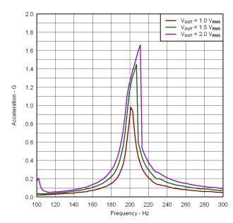
Figure 11. Acceleration Versus Frequency
