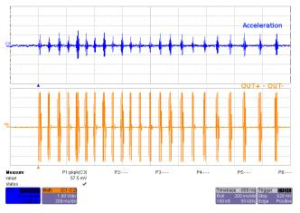
Figure 12. LRA Scroll Wheel Effect Waveform (Button 4)
