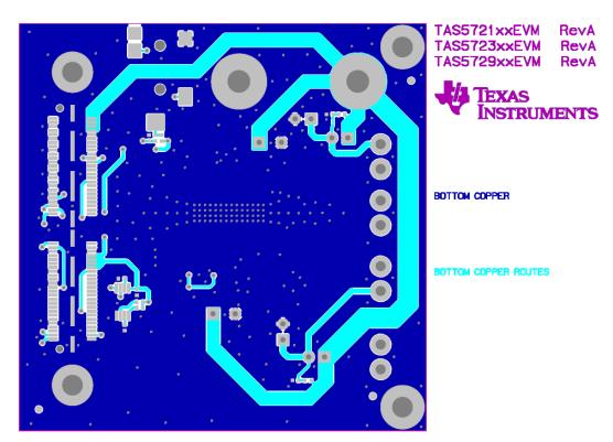
Figure 7. Bottom Copper Layout
