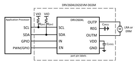
Figure 2. I<sup>2</sup>C Control with Optional PWM Input or External Trigger
