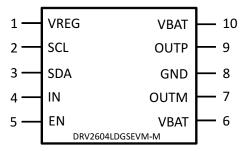
Figure 1. Pin Out of the DRV2604LDGSEVM-M
