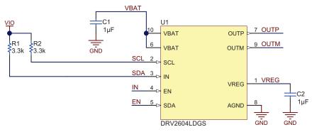
Figure 4. Schematic for the DRV2604LDGSEVM-M
