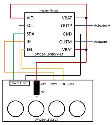
Figure 3. DRV2604LDGSEVM-M Connection to DRV2604LEVM-CT
