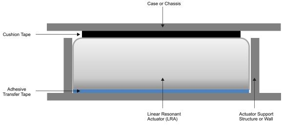
Figure 14. LRA Mounting Stack Up
