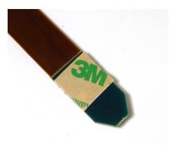
Figure 2. 3M Tape on Backside of DRV-ACC16-EVM
