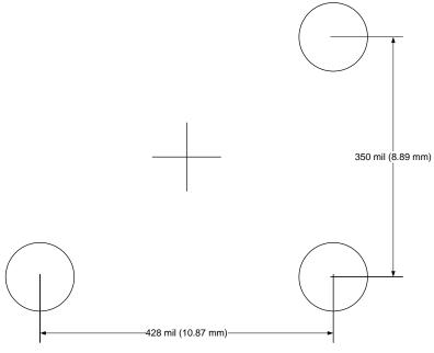
Figure 17. Screw-Hole Footprint
