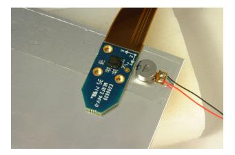
Figure 3. Attach Accelerometer to Vibrating Object
