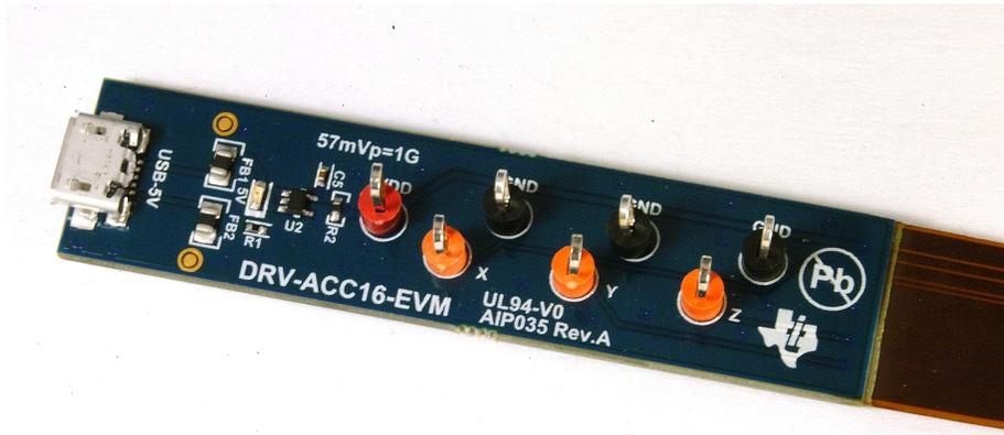
**Figure 4. DRV-ACC16-EVM - Measurement Board**
