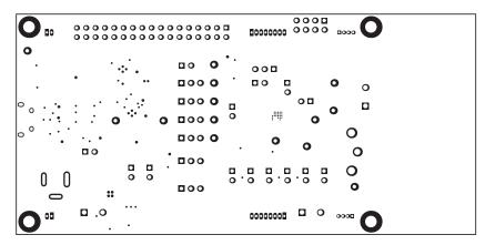
Figure 20. Bottom Solder Mask
