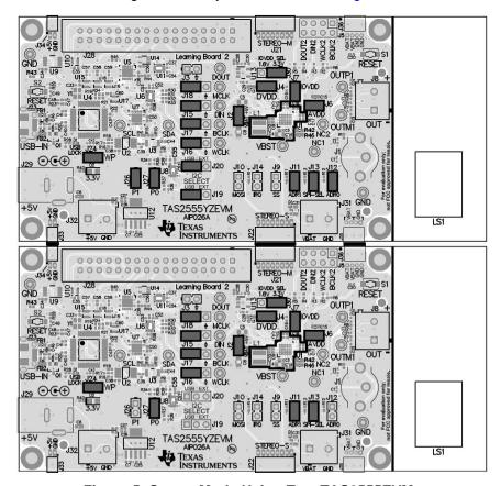
Figure 5. Stereo Mode Using Two TAS2555EVMs
