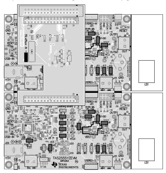
Figure 6. Stereo Adapter Board Setup
