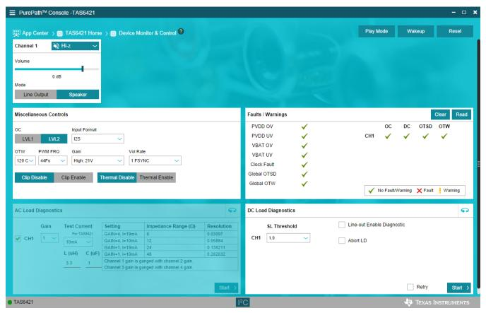
Figure 7. TAS6421-Q1 EVM Device Monitor and Control Window
