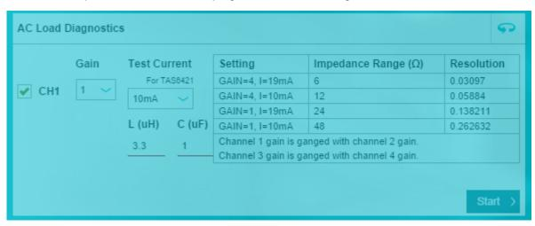
Figure 14. AC Load Diagnostics Section
