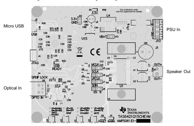
Figure 8. TAS6421-Q1 EVM Connections
