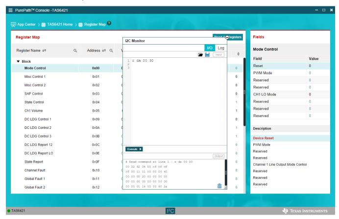
Figure 19. I2C Window - Sending I2C Commands
