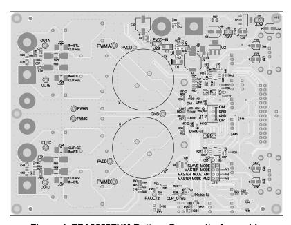
Figure 4. TPA3255EVM Bottom Composite Assembly
