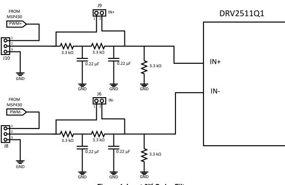
Figure 4. Input 2<sup>nd</sup> Order Filter
