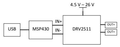
Figure 2. EVM System Block Diagram
