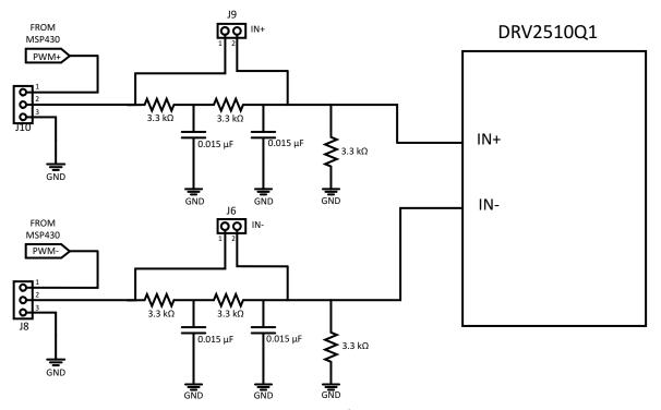
Figure 4. Input 2<sup>nd</sup> Order Filter
