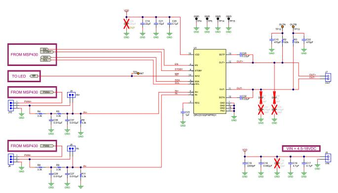
Figure 8. DRV2510Q1 Schematic 2
