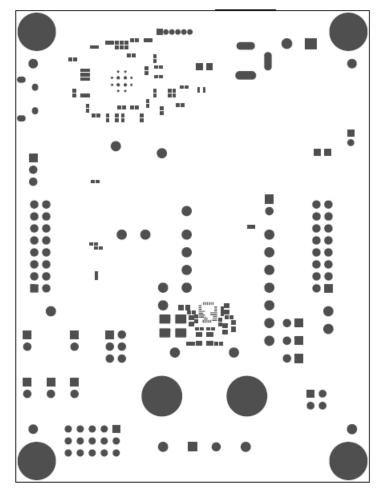
Figure 13. PCB: Top Solder Mask
