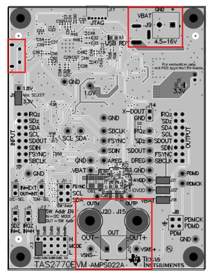
Figure 1. TAS2770EVM Stereo Configuration
