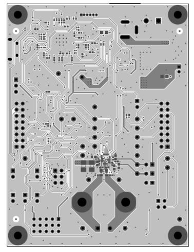
Figure 14. PCB: Top Copper
