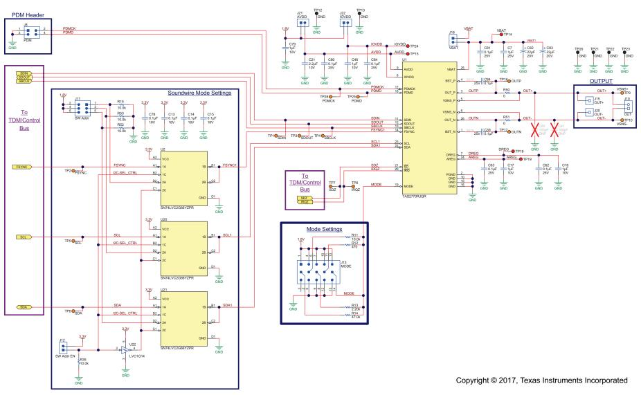
Figure 10. Schematic: TAS2770 Channel 1 Control
