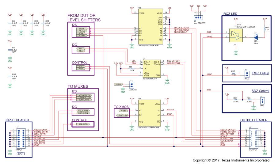
Figure 9. Schematic: External Input and Output Routing
