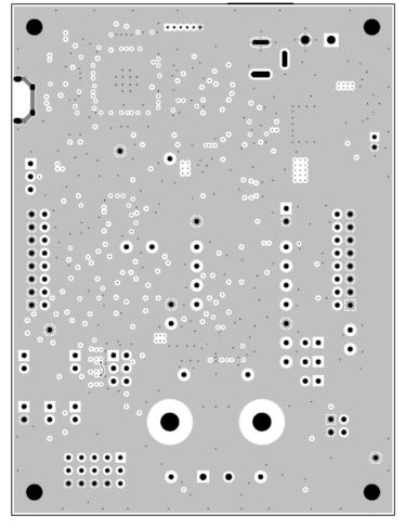
Figure 15. PCB: Copper Layer 2
