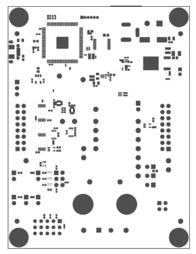
Figure 18. PCB: Bottom Solder Mask
