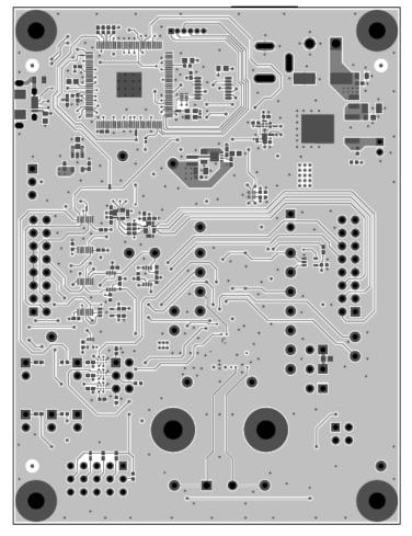
Figure 17. PCB: Bottom Copper
