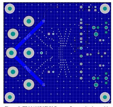
Figure 3. TPA3138D2EVM Bottom Composite Assembly
