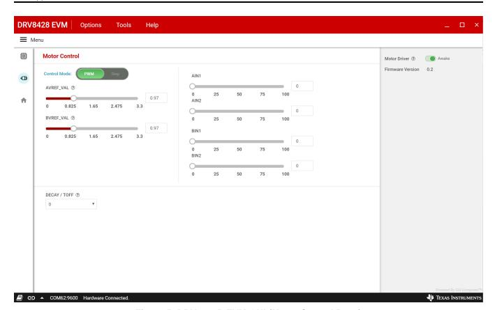
Figure 5. DRV8428P EVM GUI (Motor Control Page)
