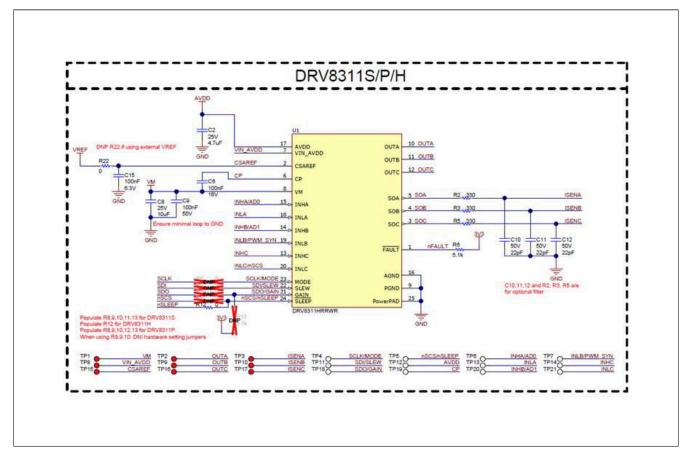
Figure 7-2. DRV8311H/S/P schematic
