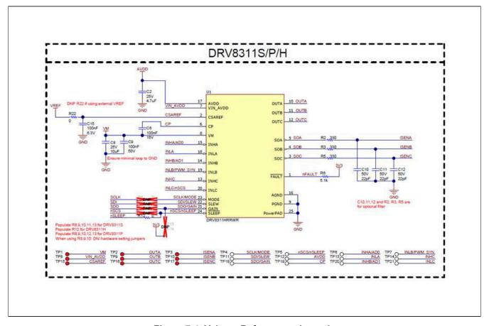
Figure 7-4. Voltage Reference schematic
