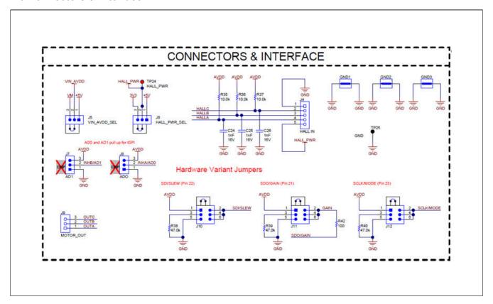
Figure 7-6. Connectors & Interface schematic
