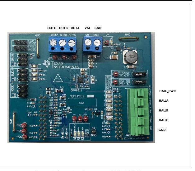
Figure 4-2. Connections from motor to DRV8311HEVM
