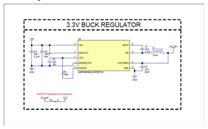
Figure 7-3. 3.3V Buck Regulator schematic
