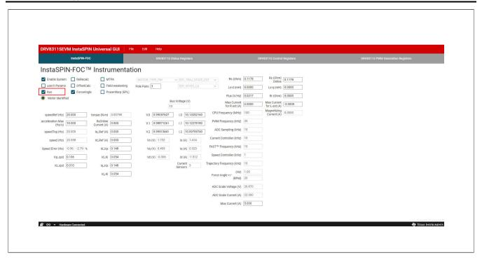
Figure 6-3. C2000 InstaSPIN Universal GUI Running motor identification
