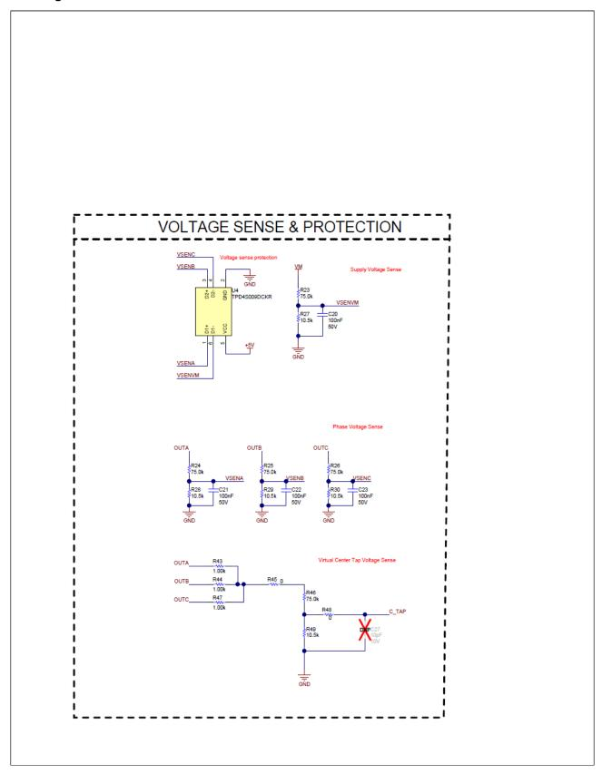
Figure 7-7. Voltage Sense & Protection schematic
