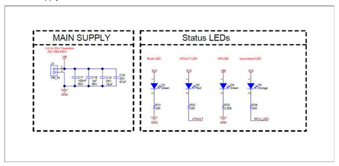
Figure 7-1. Main Supply / Status LEDs schematic
