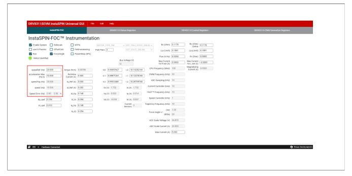
Figure 6-5. Sensorless-FOC commutation using the DRV8311HEVM InstaSPIN GUI
