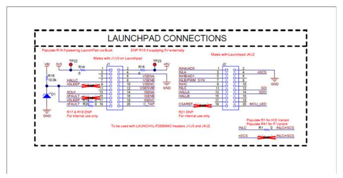
Figure 7-5. LaunchPad Connections schematic
