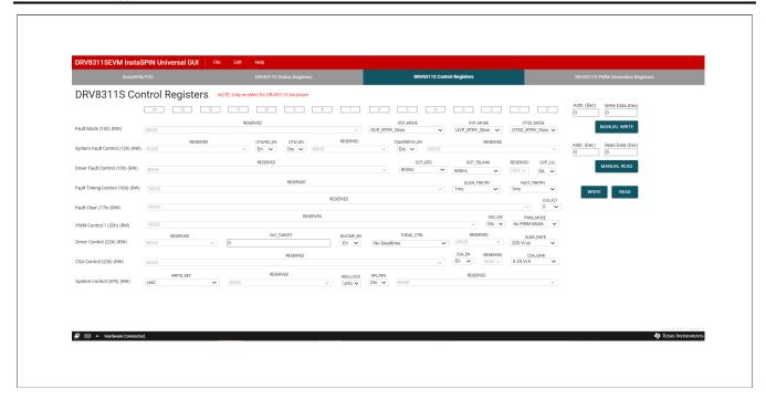
Figure 6-6. DRV8311HEVM InstaSPIN GUI SPI Control Registers
