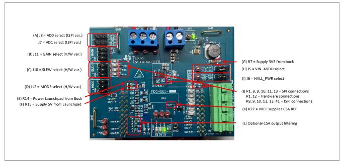
Figure 4-5. User-selectable jumpers and DNP components on DRV8311HEVM
