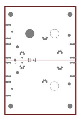
Figure 4-3. PCB Third Layer (Power)
