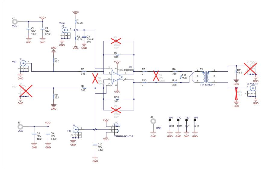
Figure 3-1. Schematic with Example Configuration Using the THS3140
