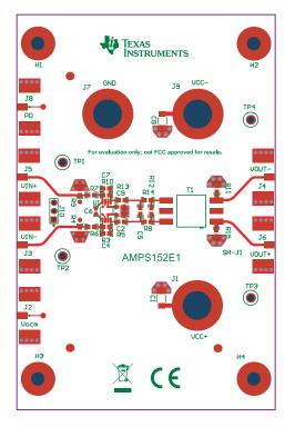
Figure 4-1. PCB Top Layers
