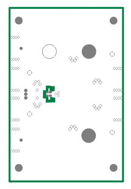
Figure 4-2. PCB Second Layer (Ground)
