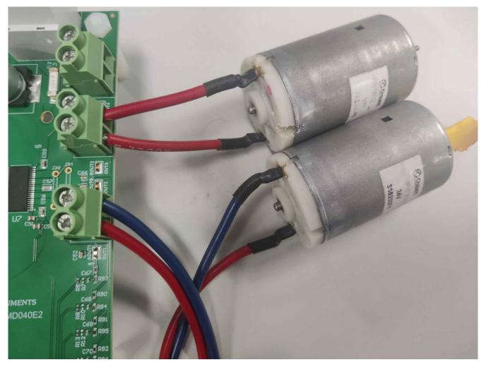
Figure 8-1. Dual motor connection to jumpers
