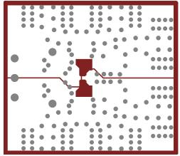
Figure 6-3. PCB Power Layer
