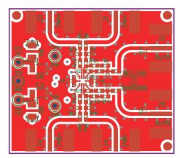
Figure 6-1. PCB Top Layers
