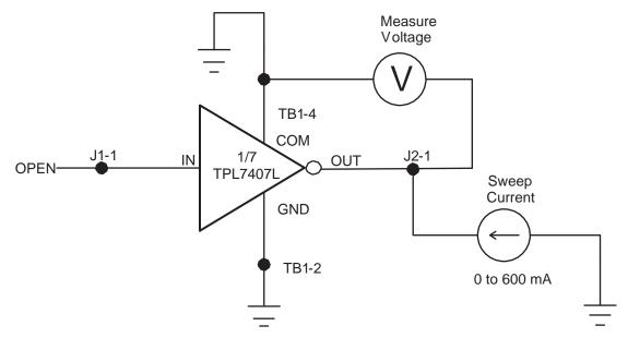
Figure 11. VF Schematic
