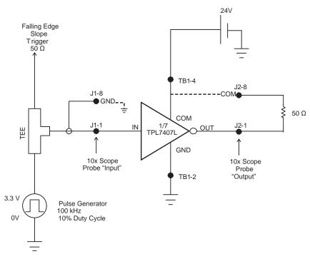
Figure 10. T<sub>PLH</sub> Schematic
