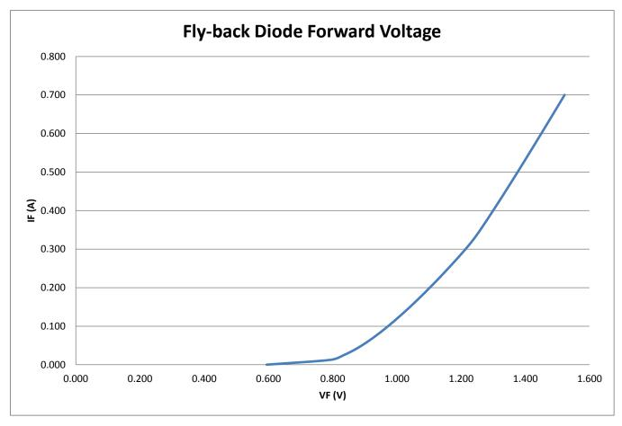
Figure 12. VF = Diode(V) vs Diode(I)
