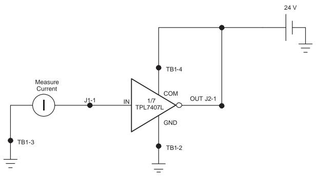
Figure 5. II(off) Schematic
