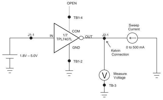
Figure 6. VOL Schematic
