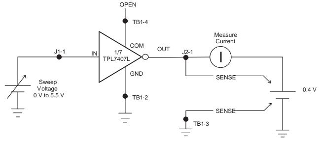
Figure 8. IOUT(on) Schematic
