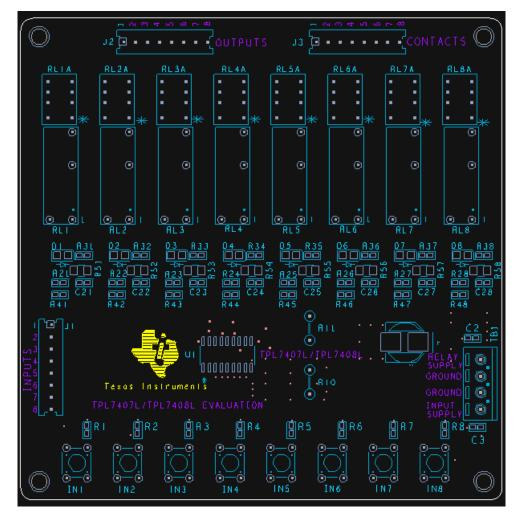
Figure 1. Physical Structure for the TPL7407LEVM (Approximate Layout)
