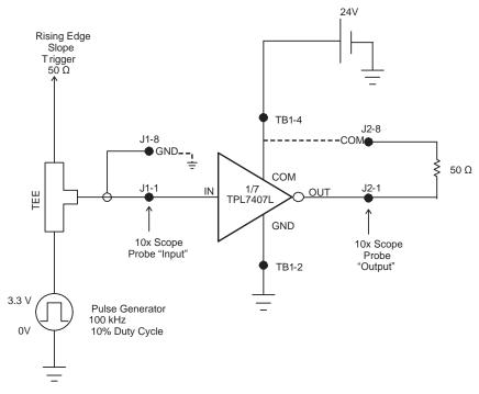
Figure 9. T<sub>PHL</sub> Schematic
