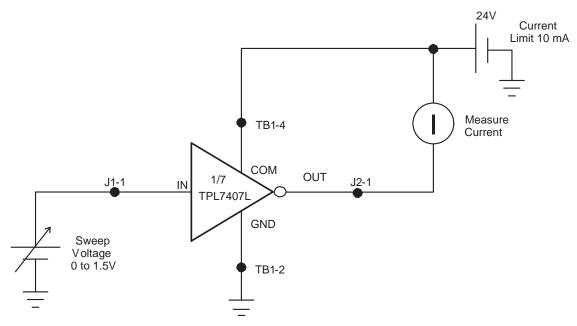
Figure 3. VI(on) and VI(off) Schematic
