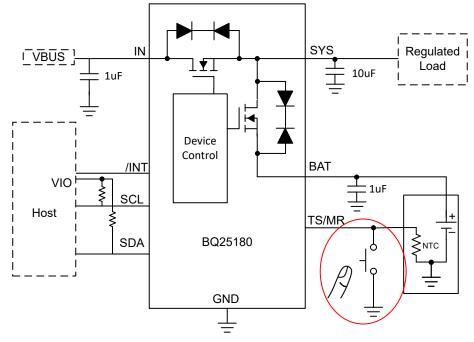
Figure 6-1. BQ25180: 1A Li-ion I2C Programmable Charger With Power Path and Ship Mode
