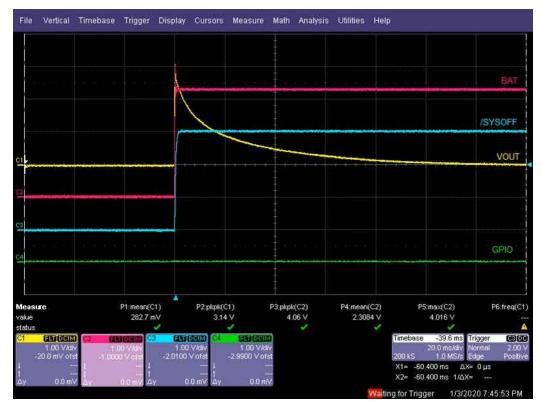
Figure 3-1. Ship Mode Upon Battery Insertion
