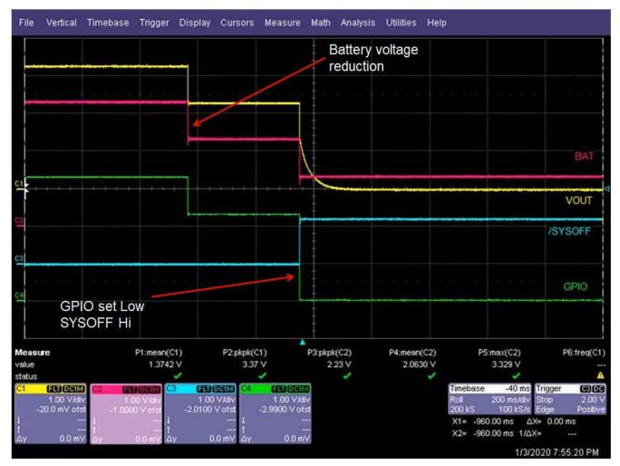
Figure 5-1. Ship Mode Reentry
