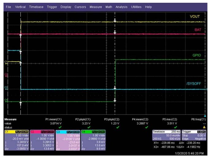
Figure 4-1. Ship Mode Exit With Push-Button
