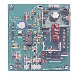
The user provides a power supply and batteries. The user configures the DV2003S2 for the number of cells,  $-\Delta V$  charge termination, and maximum charge time (with or without top-off), and commands the discharge-before-charge option with the push-button switch S1.
