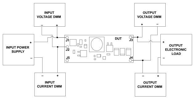
NOTES: 1. Source power should be able to supply a minimum of 0.5 A at 75 V.
