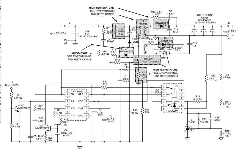
High-Voltage component. See EVM Warning and Restrictions at the back of this document. High-Temperature component. See EVM Warning and Restrictions at the back of this document.
