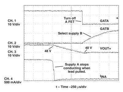
Figure 6. Switching From -48V\_INA to -48V\_INB Supply
