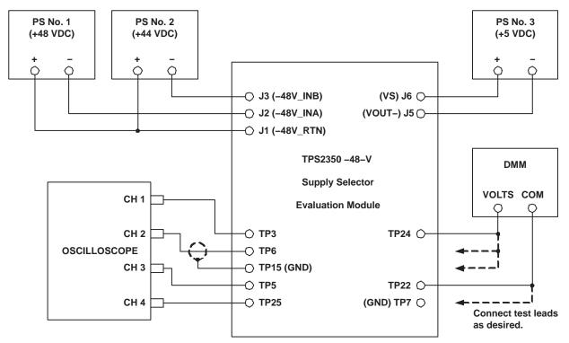
Figure 4. TPS2350 -48-V Supply Selector EVM Equipment Setup
