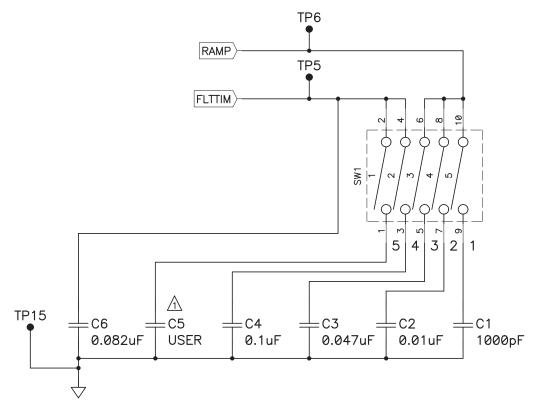
Figure 3. TPS2350 -48-V Hot Swap/Supply Selector EVM Schematic (Sheet 2)
