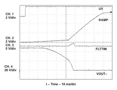
Figure 5. Load Ramp-Up Waveform
