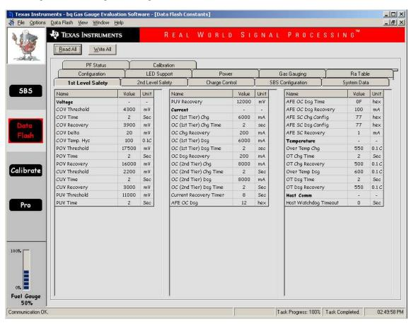
Figure 12. Data Flash Screen, 1st Level Safety Class
