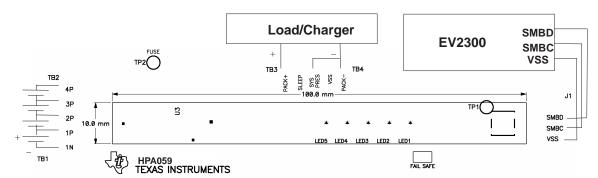
Figure 10. bq20z80bq29312 Circuit Module Connection to Cells and System Load/Charger
