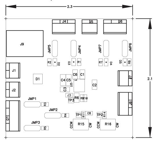
Figure 3. Top Assembly View
