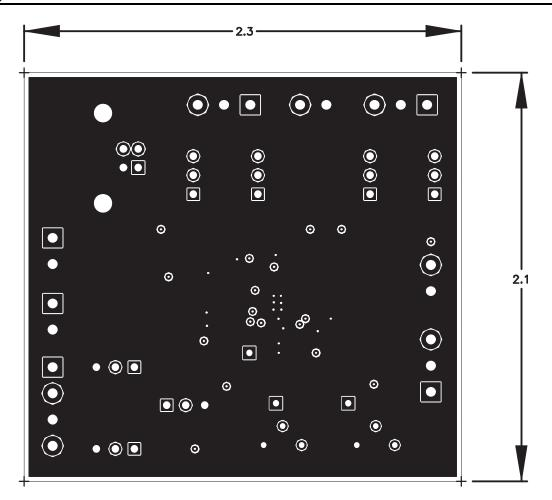
Figure 7. Board Layout - Bottom Etch Layer
