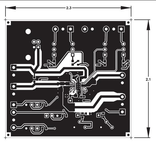
Figure 4. Board Layout – Top Etch Layer
