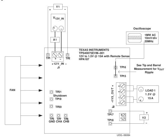
Figure 4-1. TPS40075EVM-001 Recommended Test Setup
