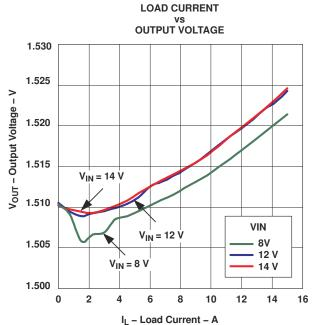
Figure 5-2. Line and Load Regulation
